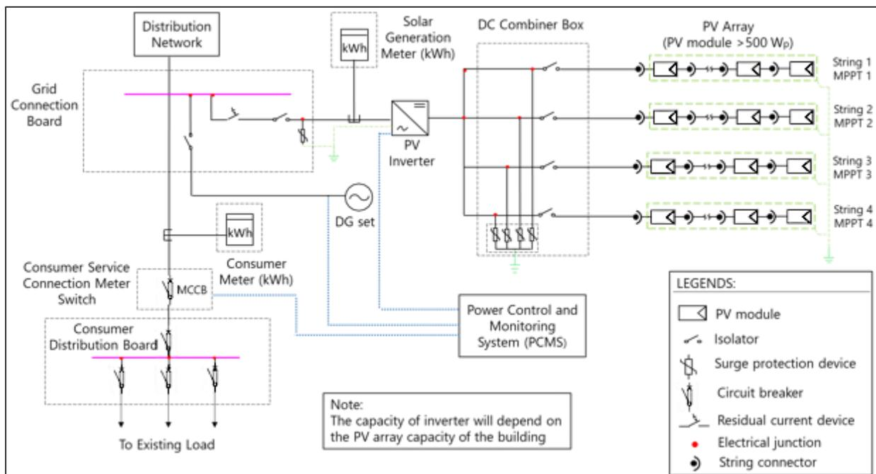
Figure 15: Single line diagram of rooftop PV system for Supremo Tribunal de Justiça (Building 2)
