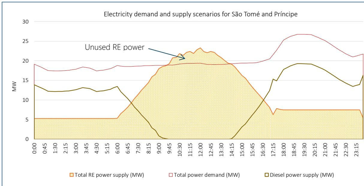
Figure 118: STP electricity demand and supply scenario (Scenario 2 – typical day)
