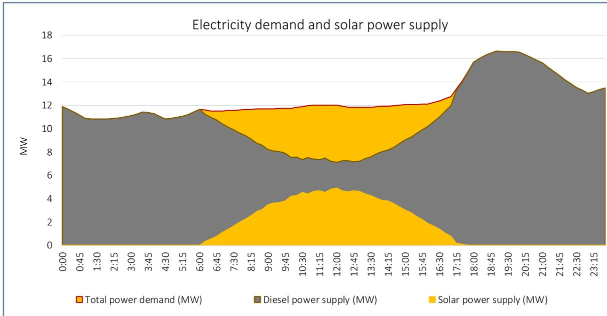
Figure 110: Typical day load profile and average solar power contribution
