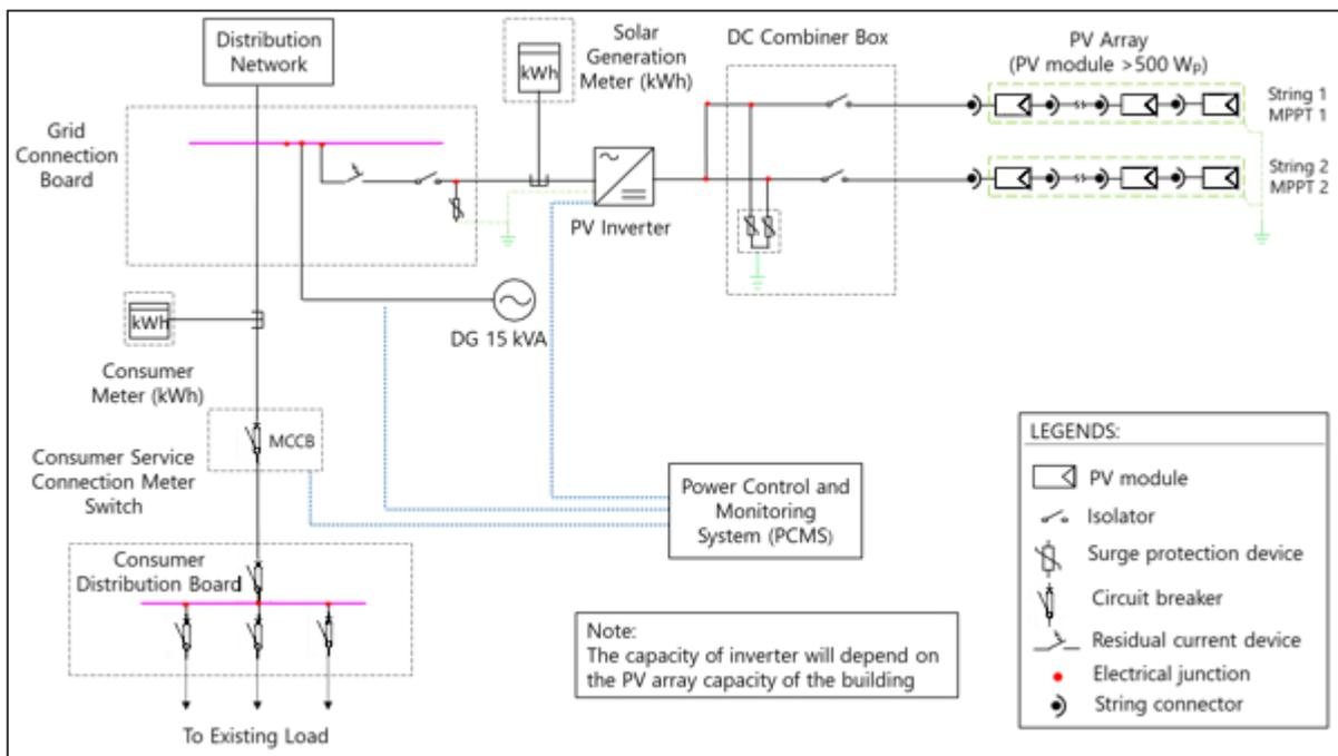
Figure 69: Single line diagram of rooftop PV system for Centro Hospitalar De Lobata
