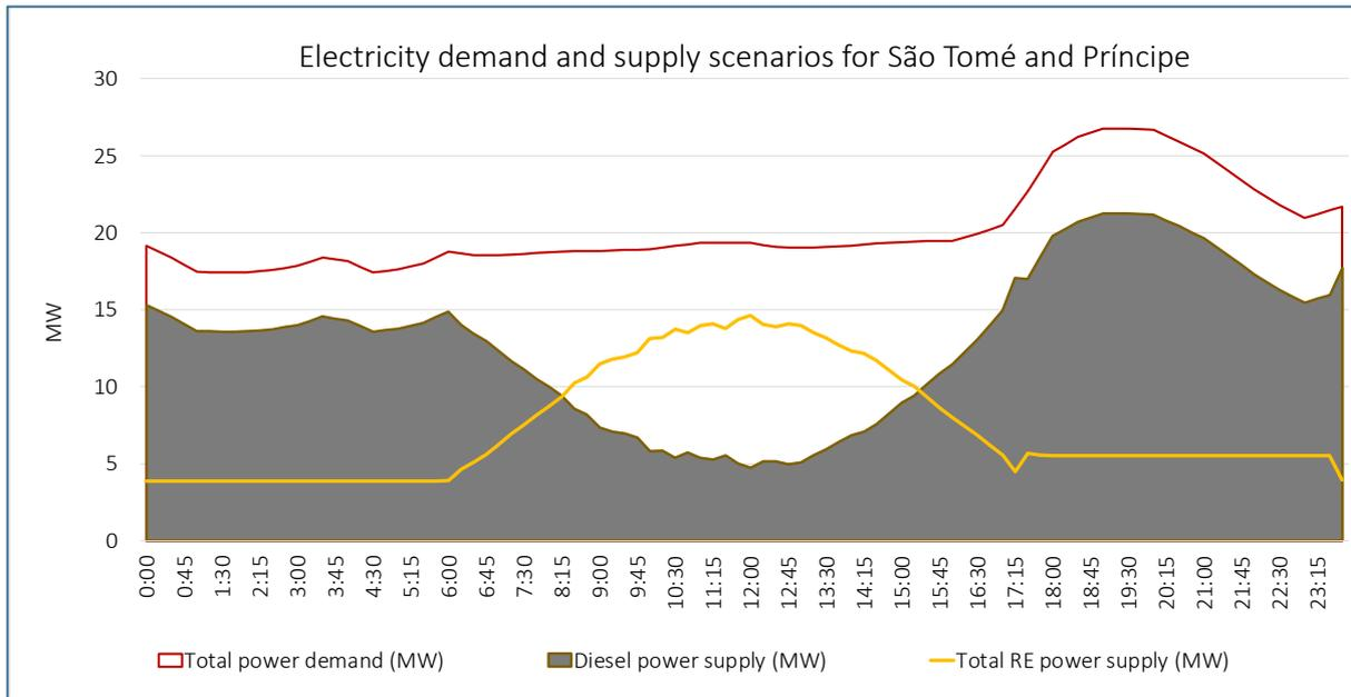
Figure 117: STP electricity demand and supply scenario (Scenario 1 – typical day)
