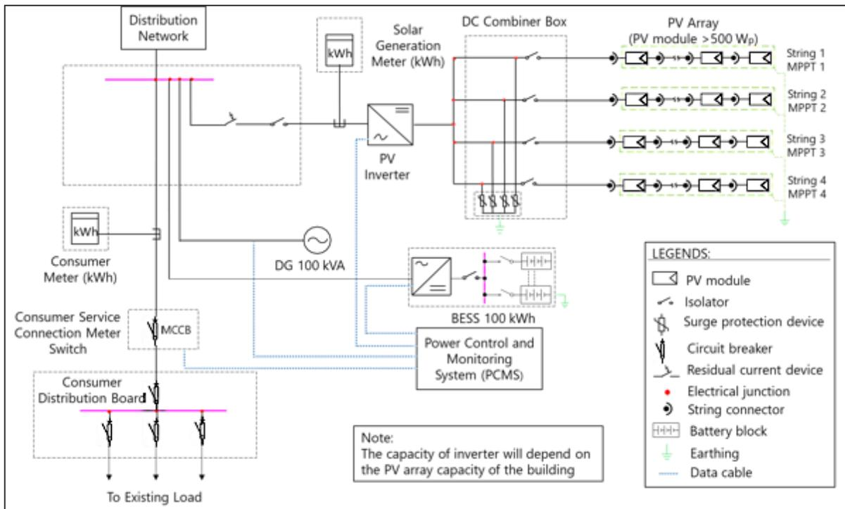
Figure 42: Single line diagram of rooftop PV system for Tribunal De Contas
