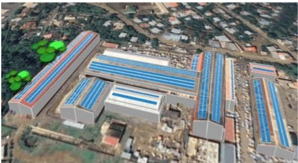
Figure 127: Site No. 15 (Mercado de Bobo Foro) with an estimated PV capacity of 937 kW<sub>p</sub>
