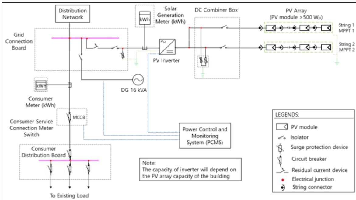
Figure 27: Single line diagram of rooftop PV system for Autoridade Geral De Regulaca (AGER)
