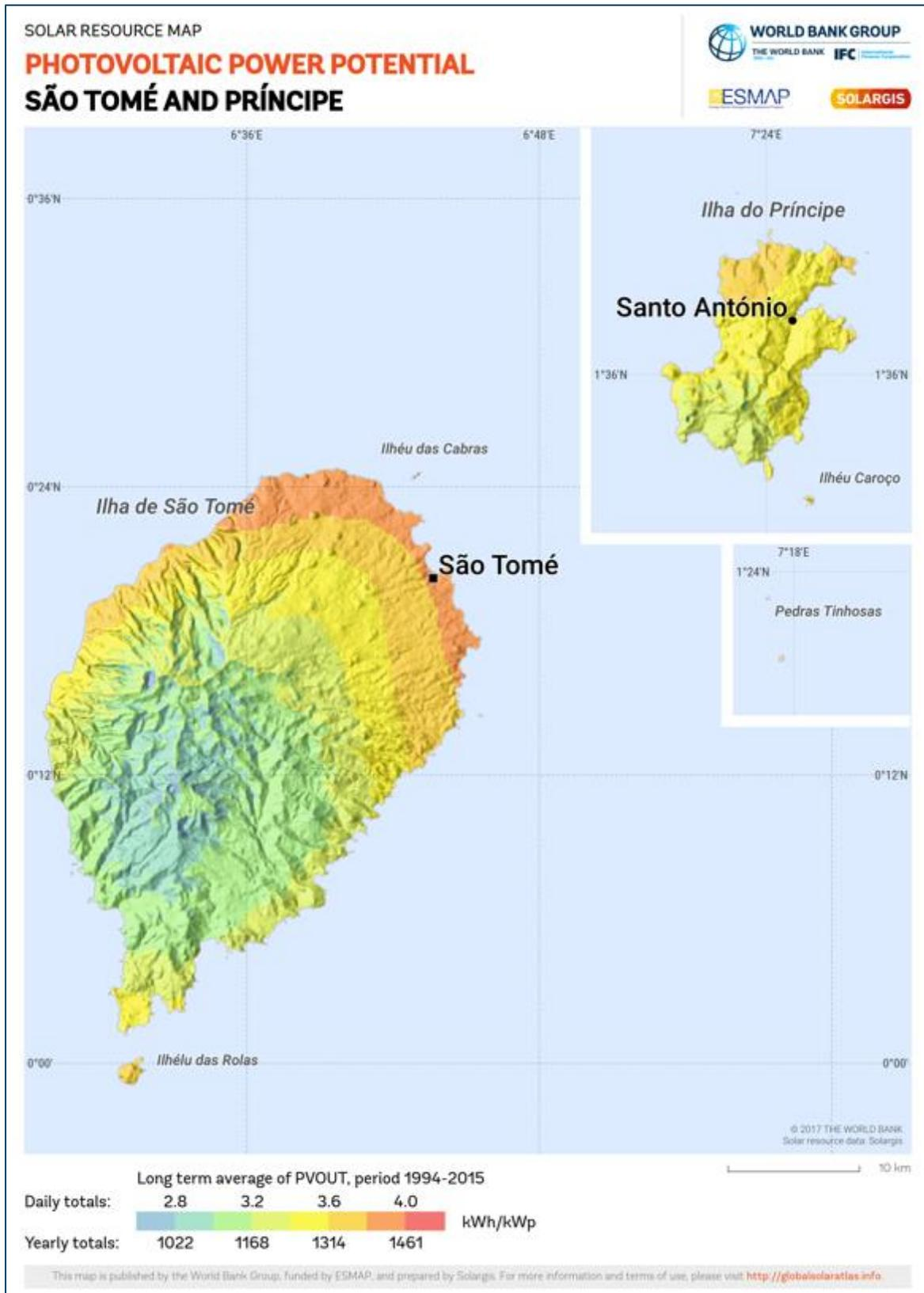
Figure 11: Solar potential in STP [<https://globalsolaratlas.info/download/sao-tome-and-principe>]
