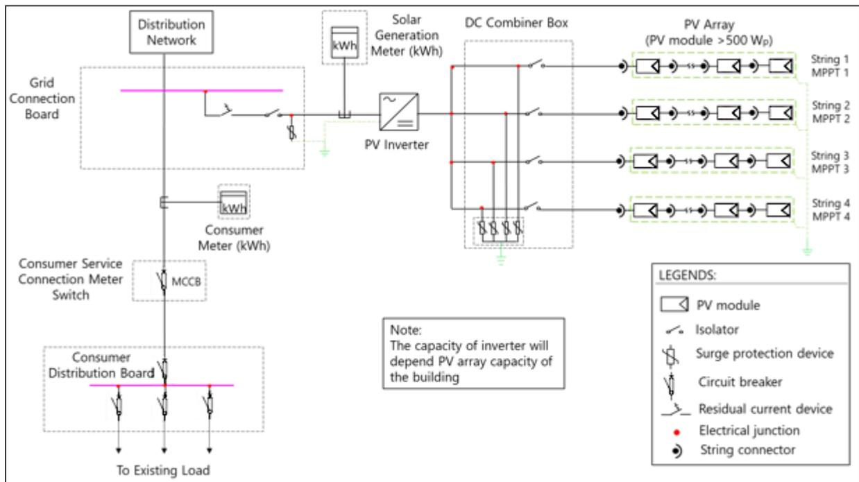
Figure 63: Single line diagram of rooftop PV system for Escola Primária De Trindade
