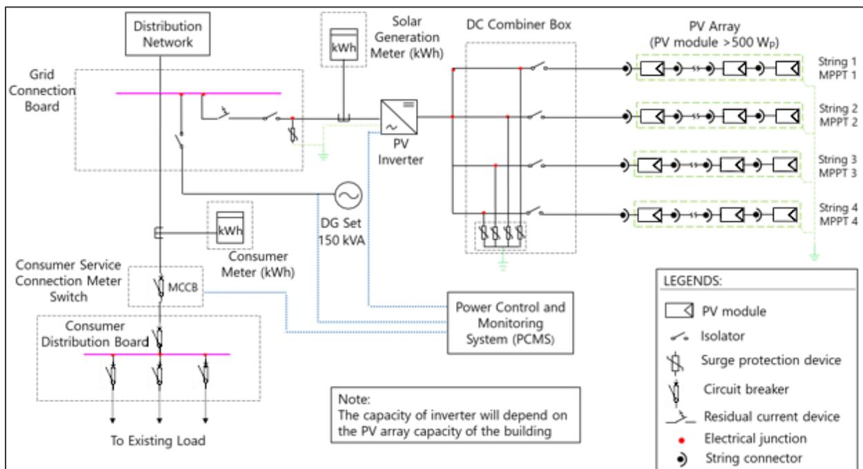
Figure 60: Single line diagram of rooftop PV system for Escola Secundaria Maria Manuela Margarido
