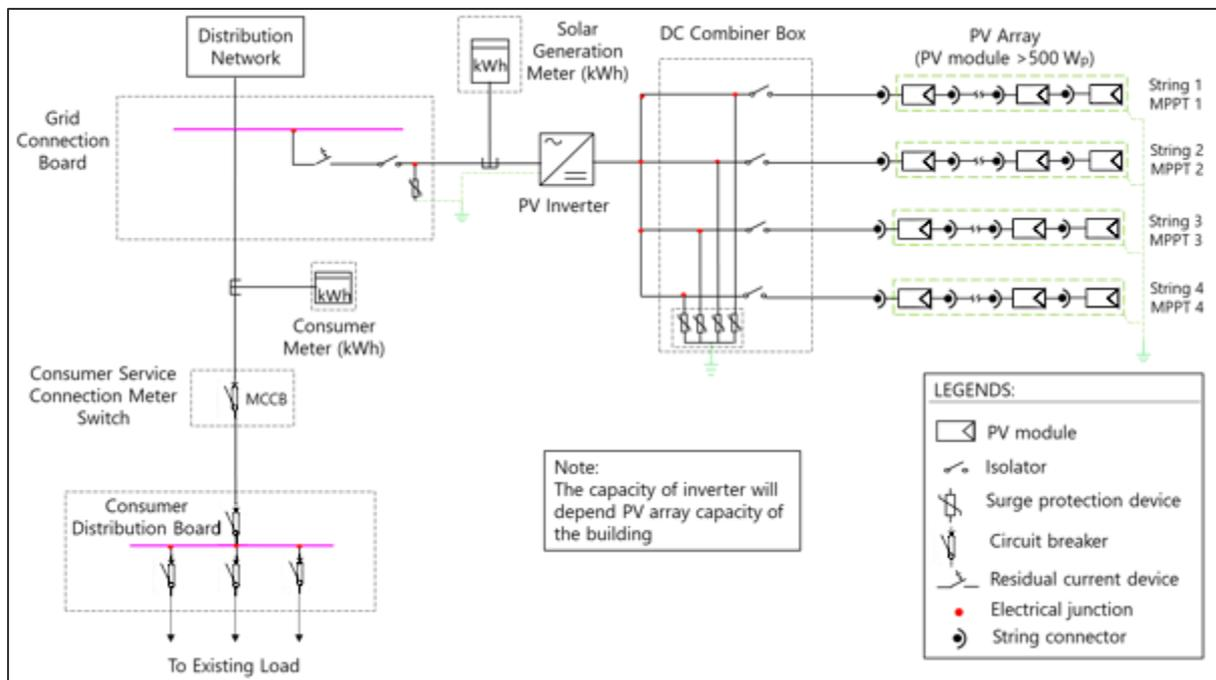
Figure 48: Single line diagram of rooftop PV system for Centro Polivalente De Caué
