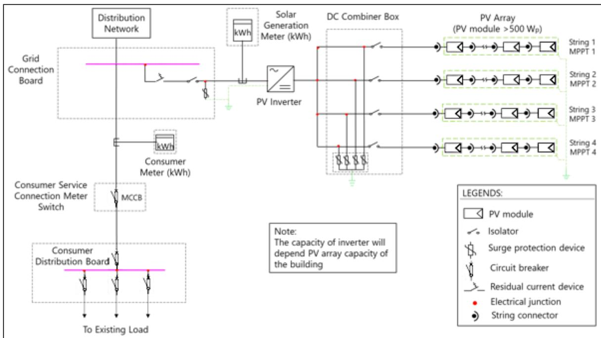
Figure 45: Single line diagram of rooftop PV system for Liceu Nacional De Santana
