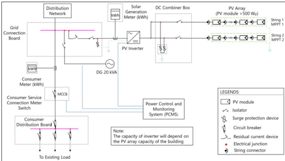
Figure 21: Single line diagram of rooftop PV system for Procurador/Ministério Público
