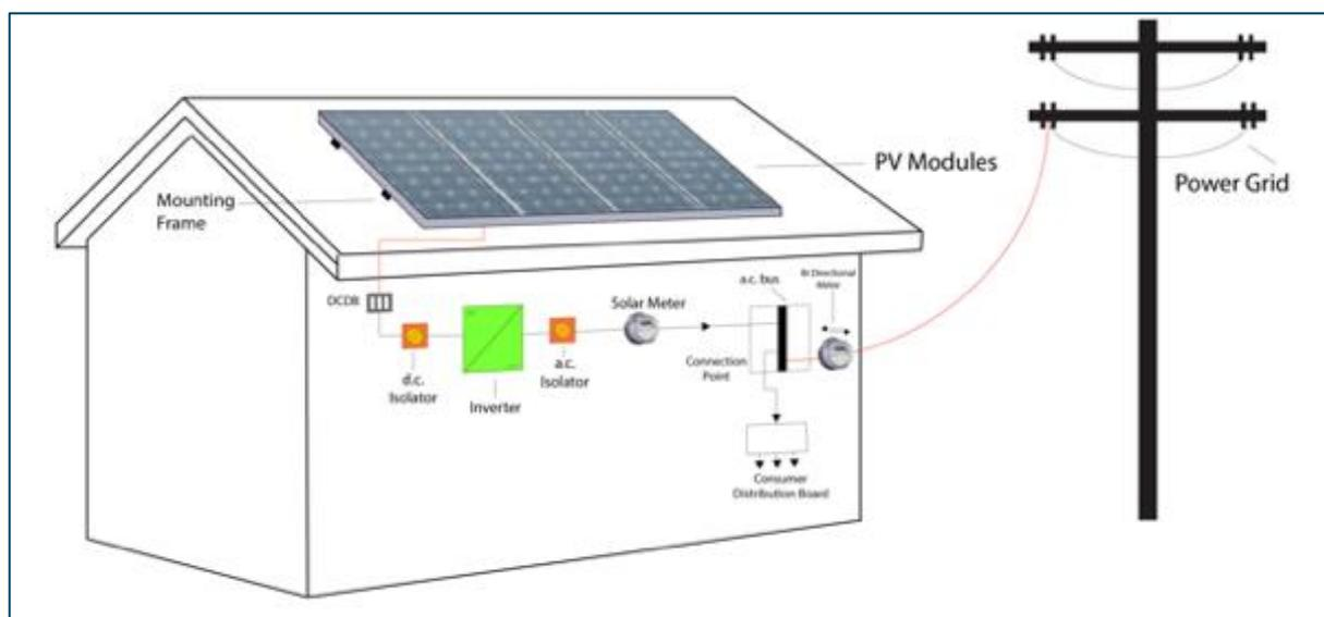
Figure 129: Net metering arrangement
