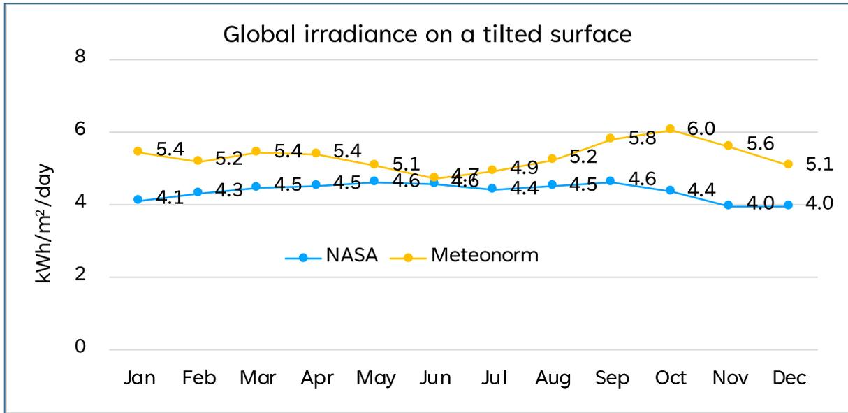
Figure 10: Global irradiance on a tilted surface in kWh/m<sup>2</sup>/day
