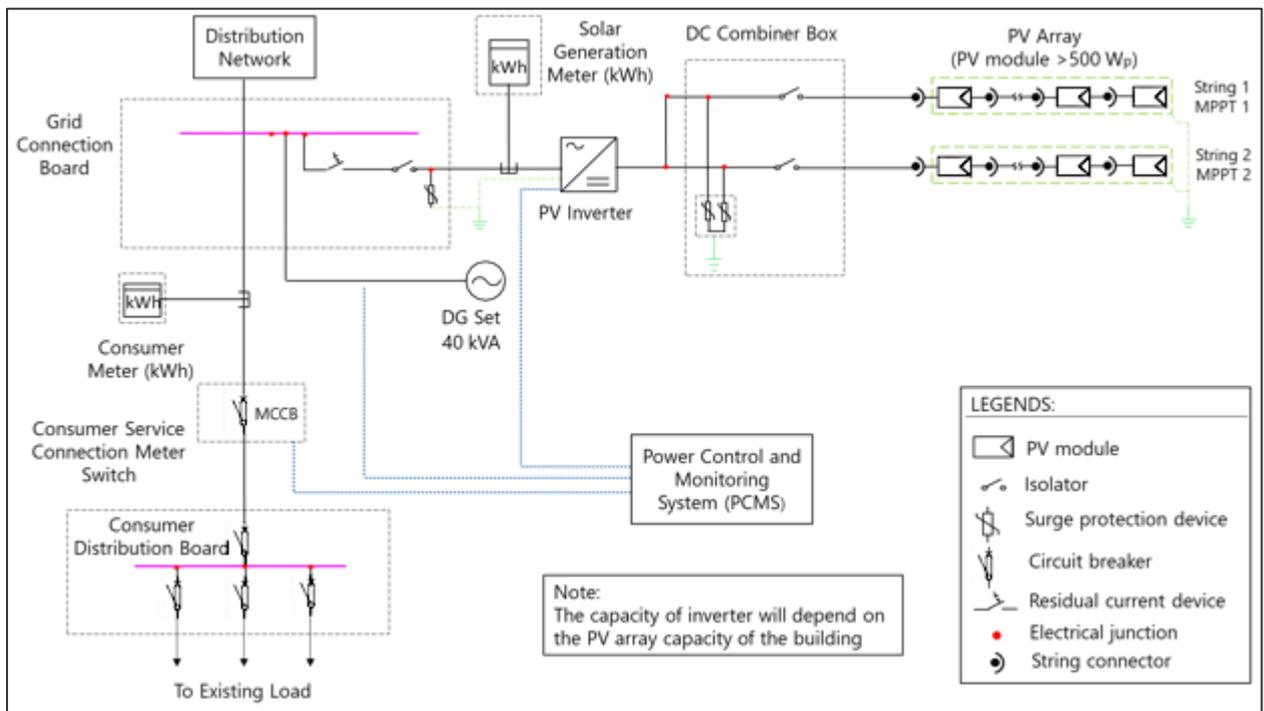
Figure 72: Single line diagram of rooftop PV system for Camara Distrital De Lobata
