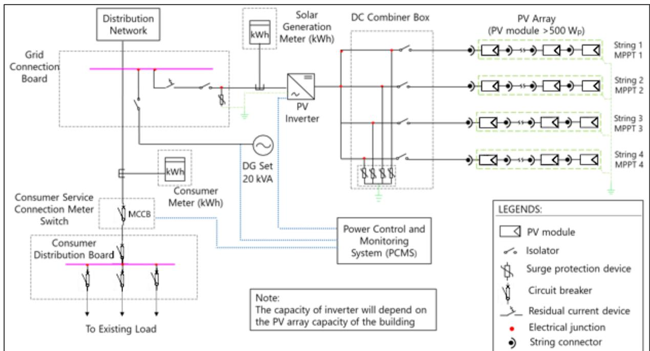
Figure 54: Single line diagram of rooftop PV system Posto De Saúde
