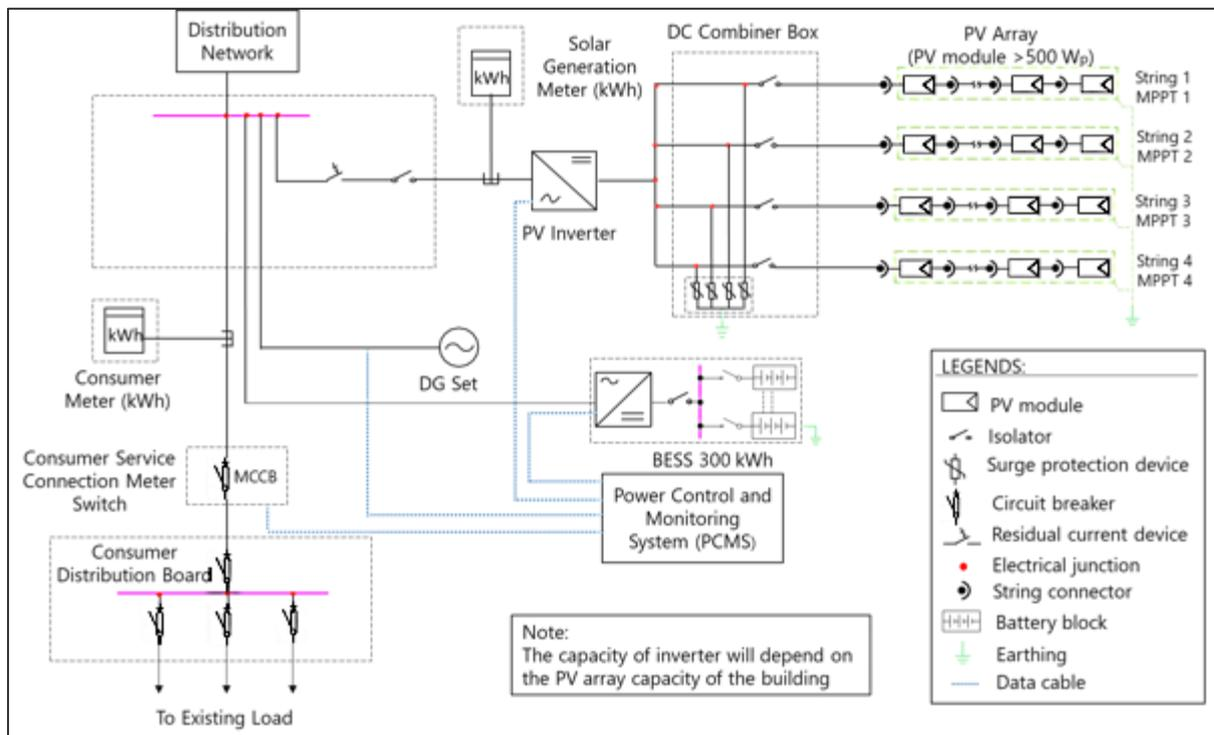
Figure 98: Single line diagram of rooftop PV system for Banco Internacional De São Tomé & Príncipe
