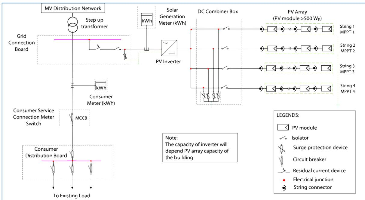
Figure 57: Single line diagram of rooftop PV system for Mercado De Bobo Foro
