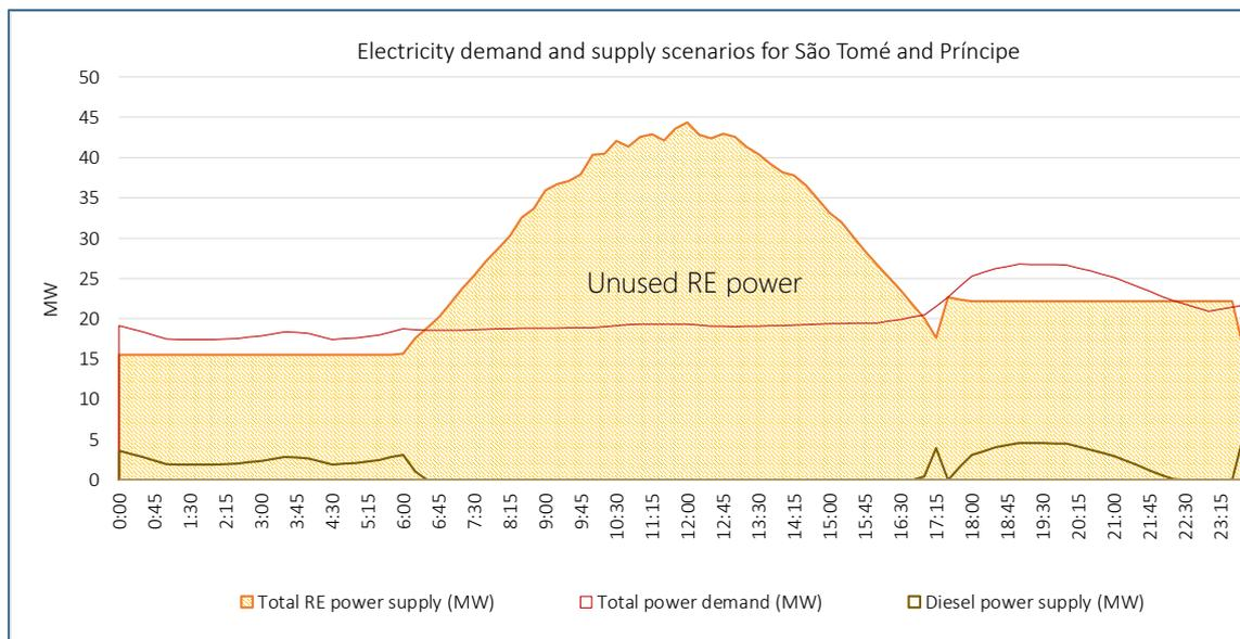
Figure 119: STP electricity demand and supply scenario (Scenario 3 – typical day)
