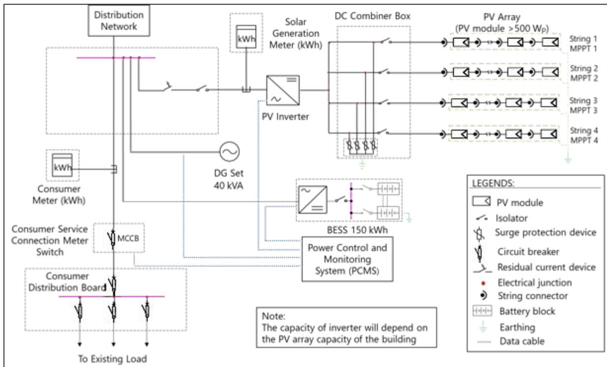
Figure 107: Single line diagram of rooftop PV system for Hospital Dr. Manuel Quaresma Dias da Graça
