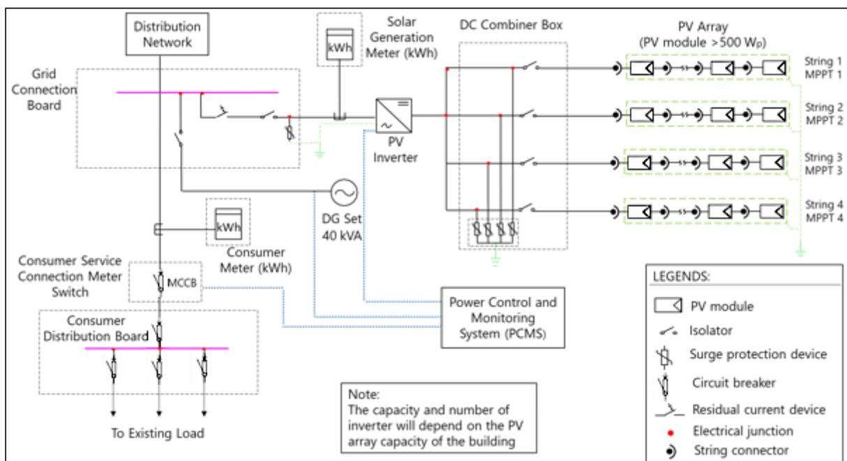
Figure 36: Single line diagram of rooftop PV system for Liceu Nacional
