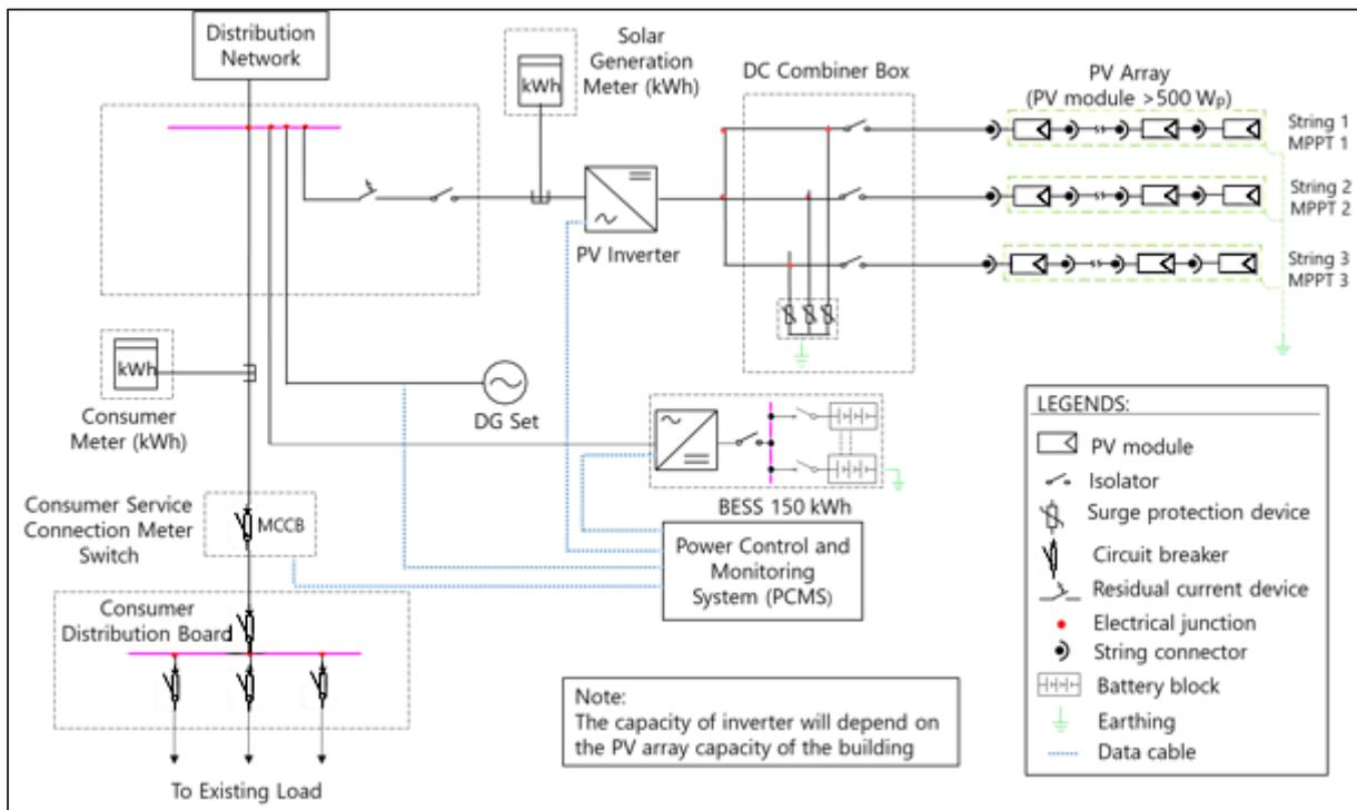
Figure 89: Single line diagram of rooftop PV system for Fabrica De Chocolate
