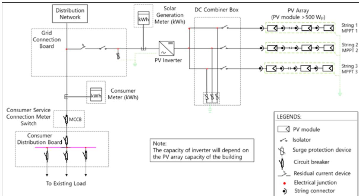
Figure 86: Single line diagram of rooftop PV system for Camara Distrital De Lembá
