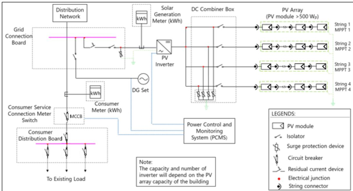
Figure 30: Single line diagram of rooftop PV system for Hospital Dr. Aires De Menezes
