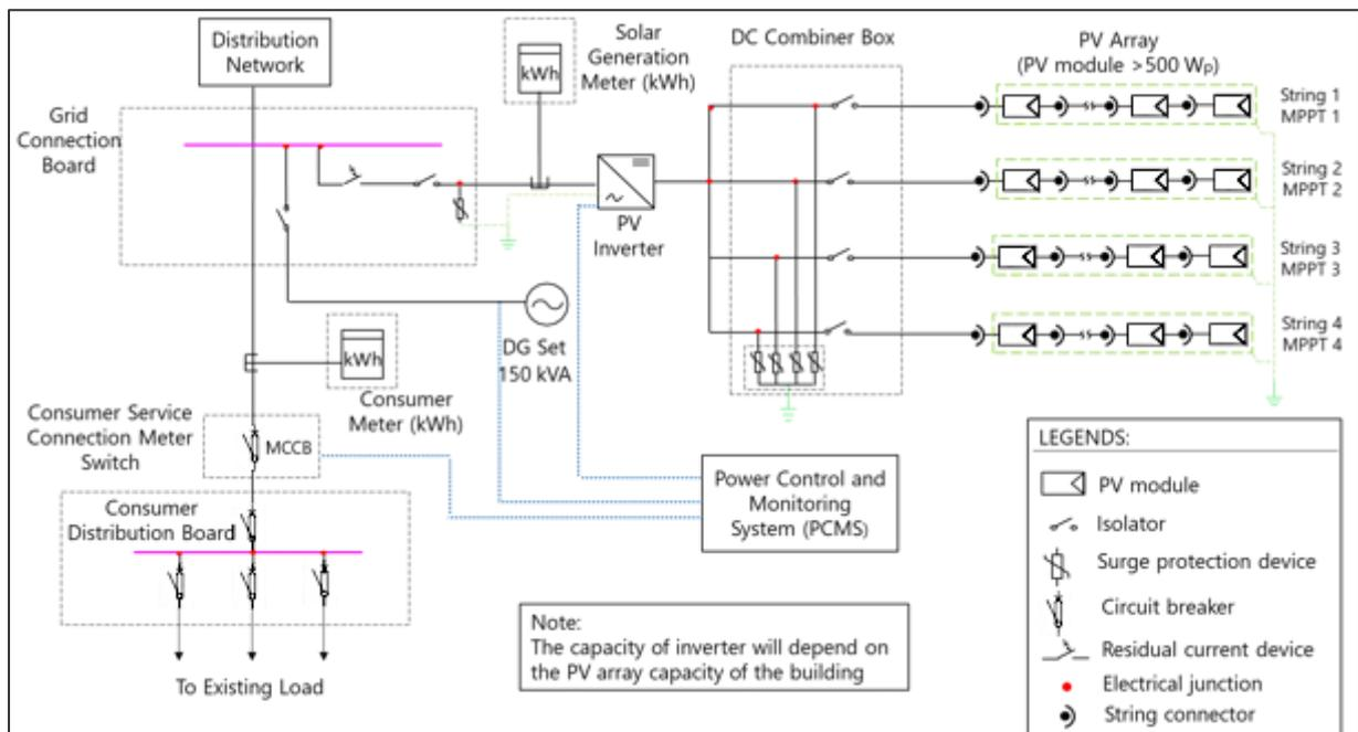
Figure 66: Single line diagram of rooftop PV system for Liceu Mé Chinhô
