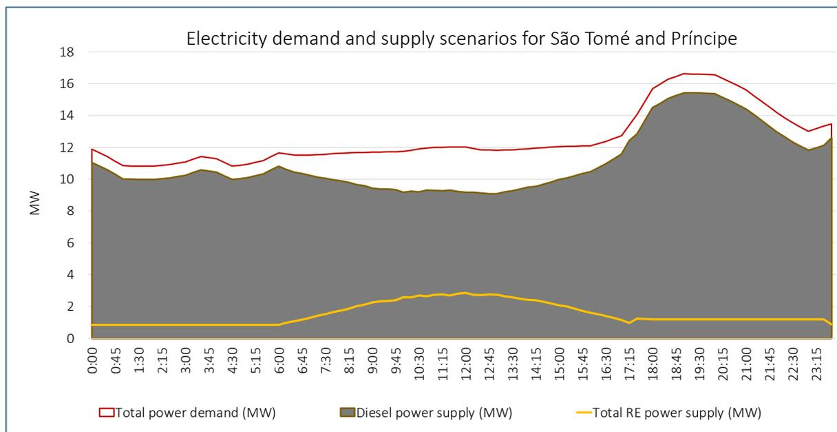
Figure 116: STP electricity demand and supply scenario (Base case – typical day)
