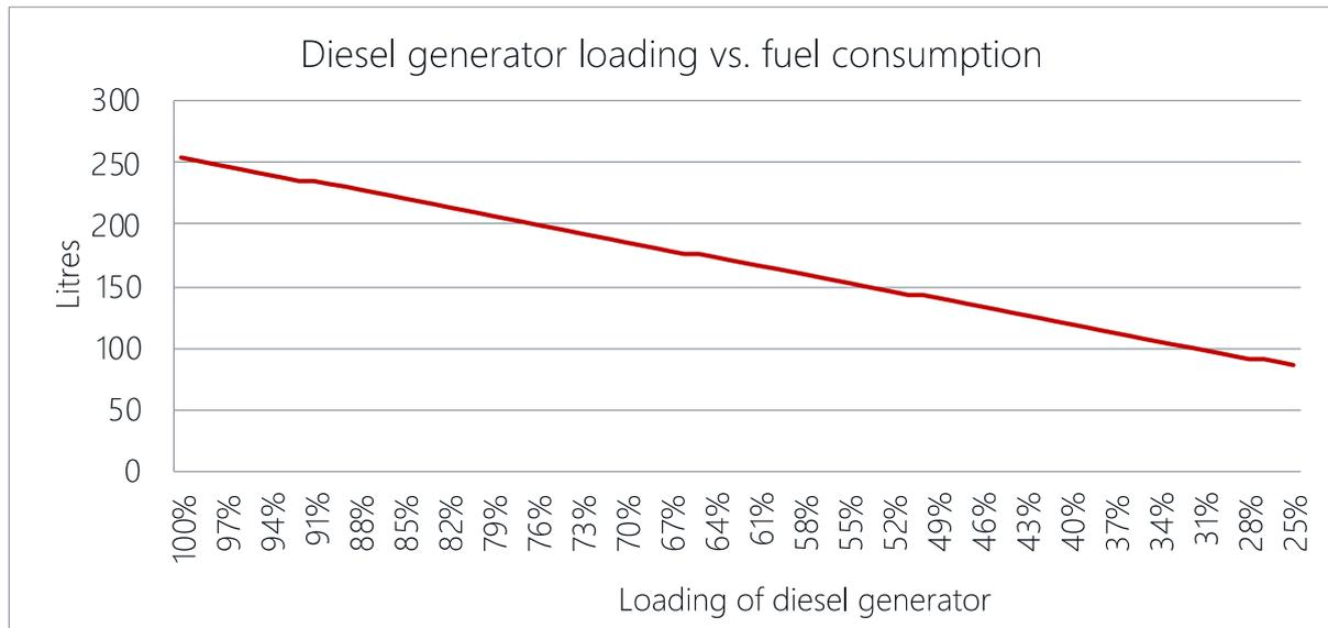
Figure 109: Diesel generator fuel consumption vs loading (1 MW plant) (Source: Caterpillar)
