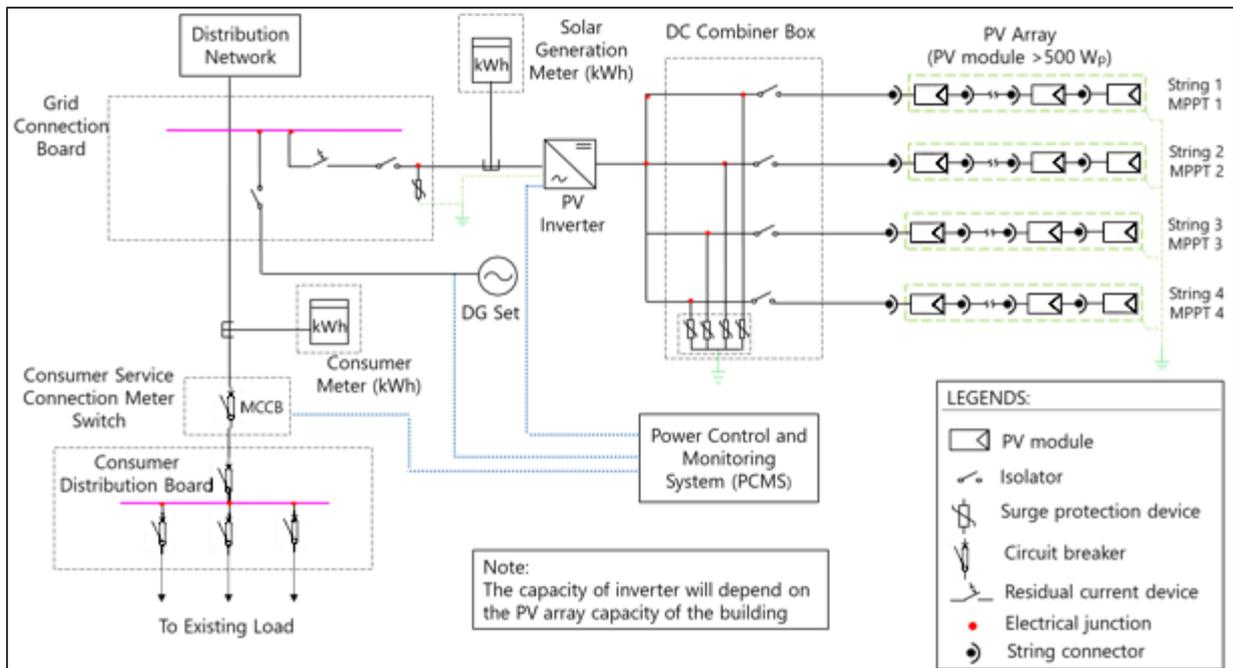
Figure 24: Single line diagram of rooftop PV system for Ministério Da Defesa
