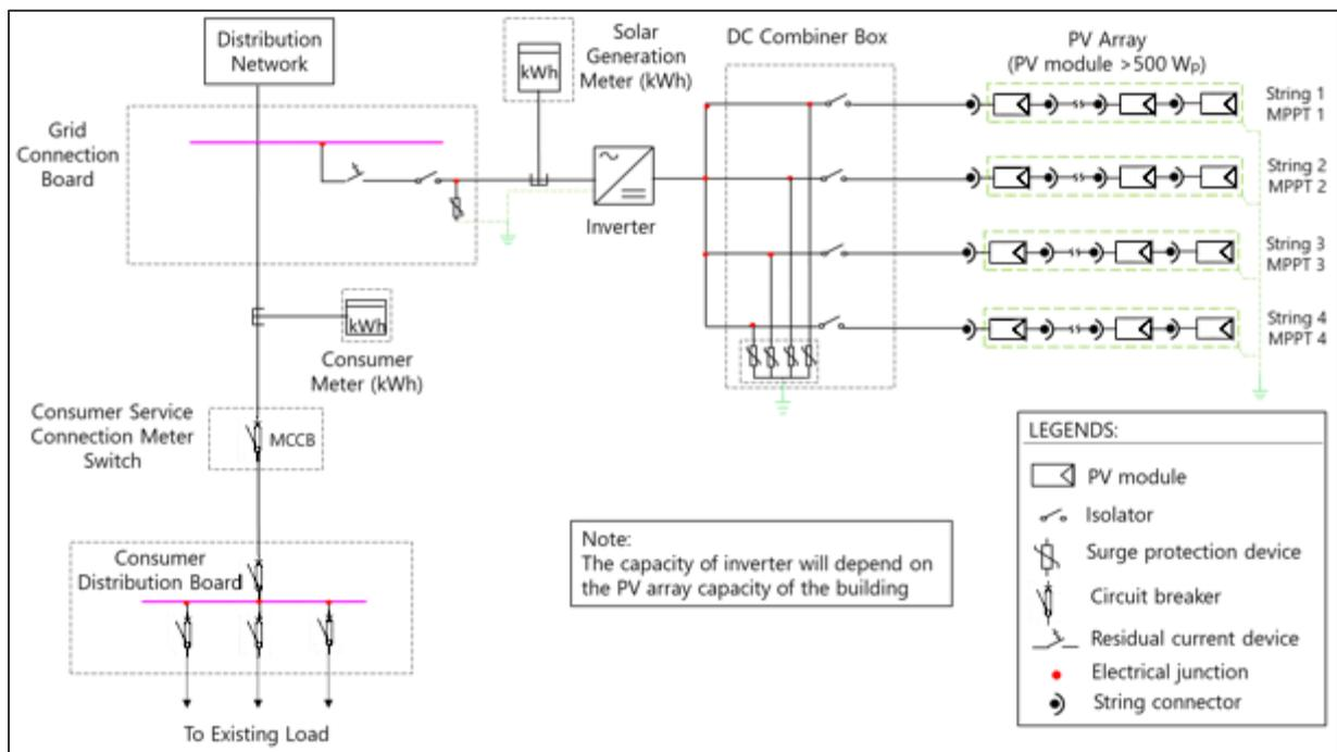
Figure 75: Single line diagram of rooftop PV system for Escola Secundária De Neves
