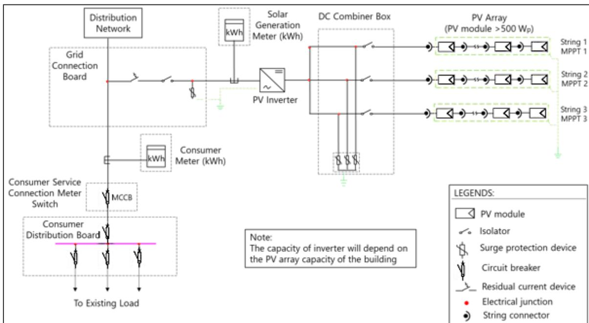
Figure 81: Single line diagram of rooftop PV system for Posto De Saude De Lembá
