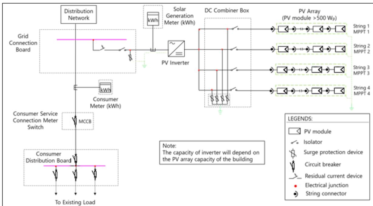
Figure 95: Single line diagram of rooftop PV system for Escola De Padrão
