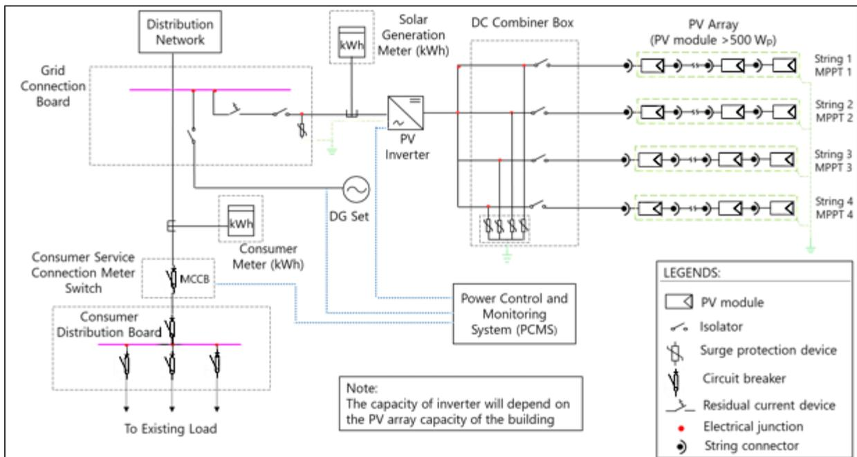
Figure 101: Single line diagram of rooftop PV system for Casa Da Cultura
