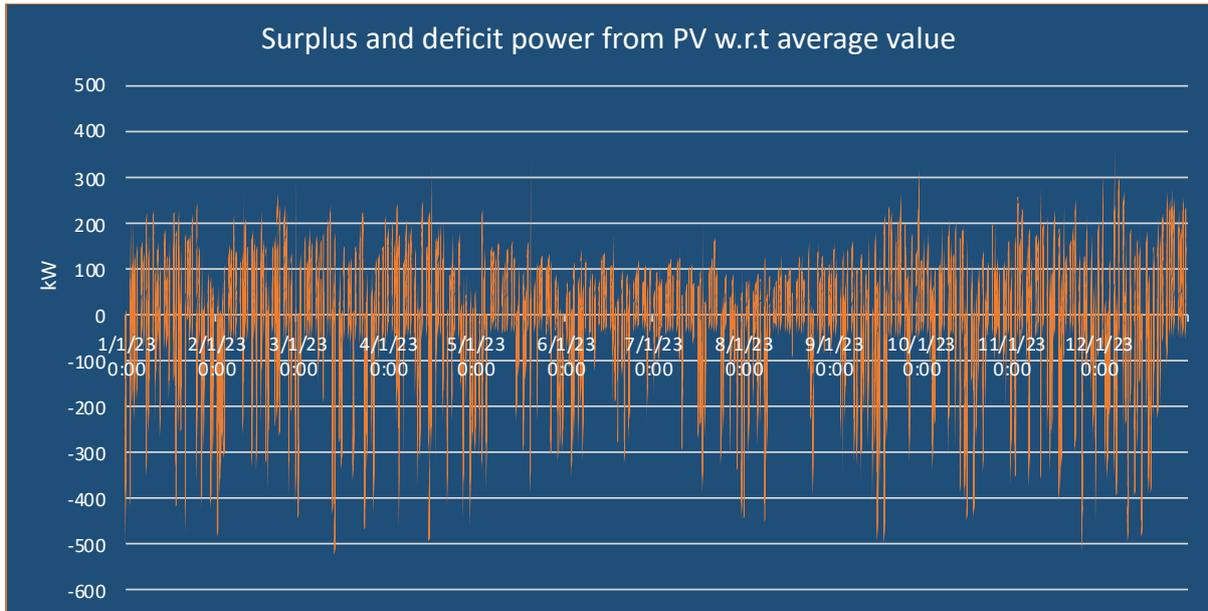
Figure 113: Surplus and deficit power from 1 MW<sub>p</sub> PV power plant w.r.t average value
